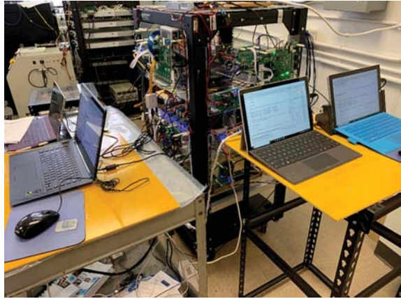
Figure 8.13 A photo of the one-phase AC/DC microgrid test-bed under development. Source: Yinliang Xu.
