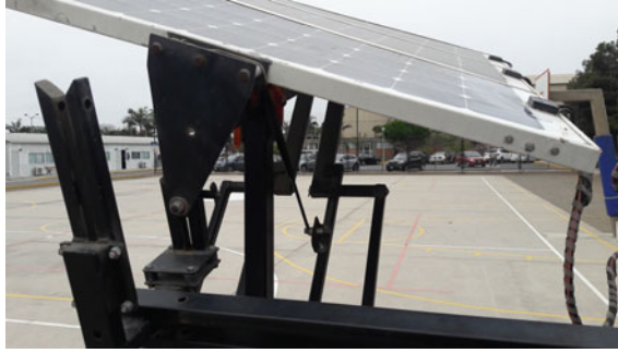
Fig. 21.4 Detail of the solar tracker mechanism, which consists of a modified slider crank mechanism: The bottom black bar is the slider and the triangular plate is the crank, connected to the solar panel
