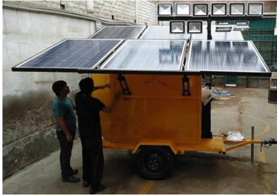
Fig. 21.2 First prototype of the mobile illumination tower
