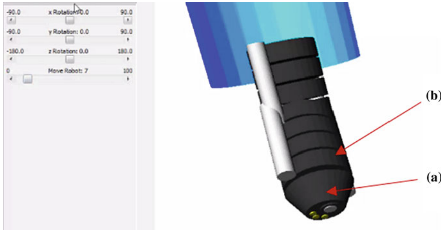
Fig. 7.3 Representation of the Flex@ Drive, in MobileBody SDK; a represents the head/endoscope (spherical joint) and b represents one section of the snake-like body (revolute joint) that follows the manipulator's head. On the left side, one can see the scrollbars that control each variable of the head. Rotation around the X, Y, and Z Axes and "Move Robot" that allows the robot's body to move forward and to retract to a previous position (backward)
