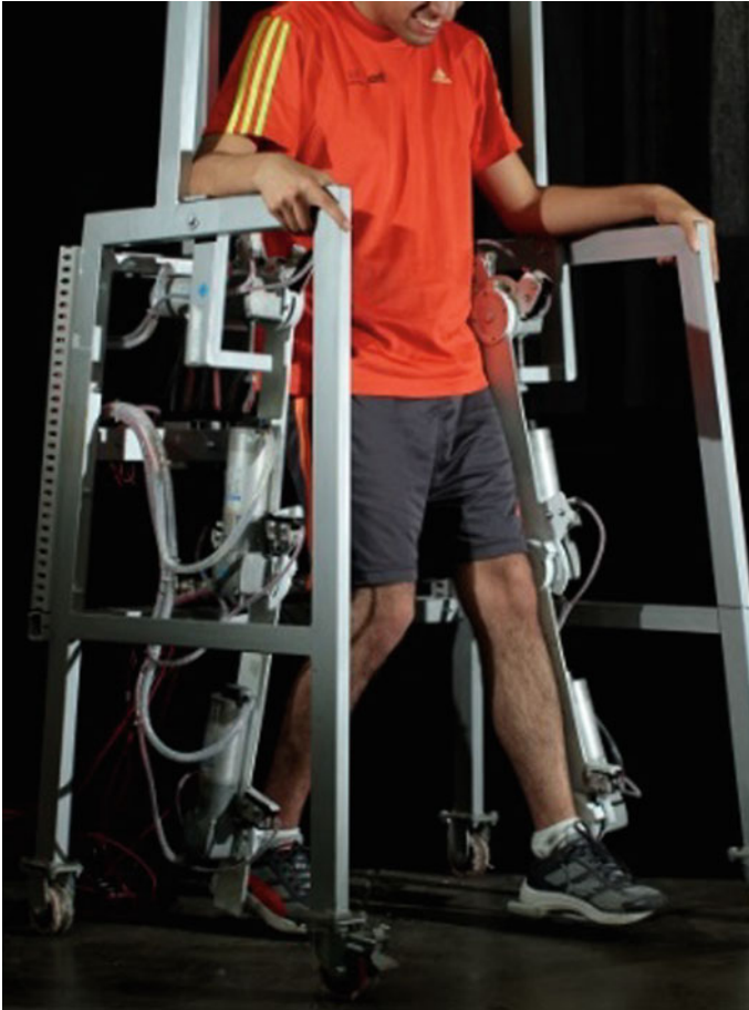
Fig. 8.7 Lima lower limb exoskeleton robotic system prototype. The figure shows how a user should be positioned in the prototype. The prototype has not been yet tested with actual human subjects
