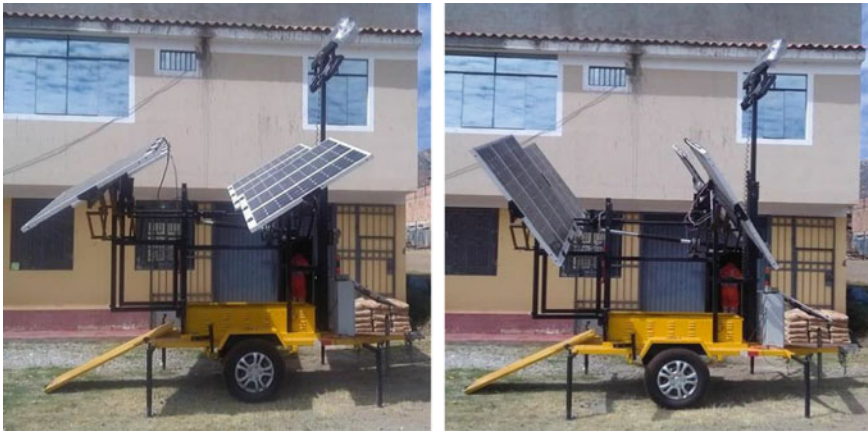
Fig. 21.3 Second and improved prototype, showing its solar tracking mechanism in different positions at 8 am (left) and 4 pm (right) during a field test in the Peruvian highlands
