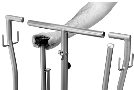
FIGURE 19.4 Arm rise and fall control. Photos courtesy of J. L. Fisher, Inc.
