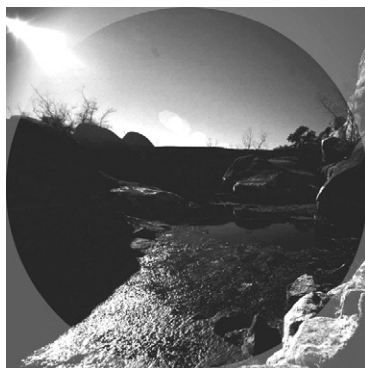
FIGURE 29.4 An image circle covering a circle of diameter of about 1.785 inches or 45.33 mm.
