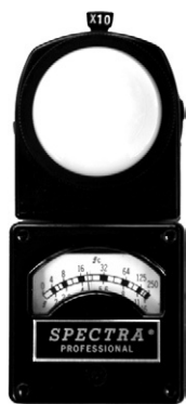
FIGURE 24.8 Spectra professional light meter (P-251 Classic). Reproduced by permission of Spectra Cine, Inc.
