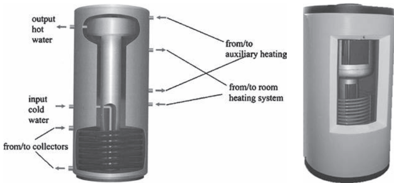
Figure 67: Tank in tank storage tank.
