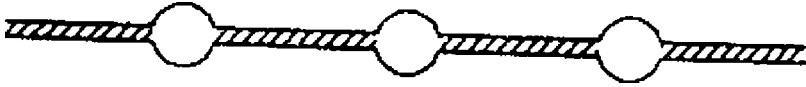
Figure 8: Pipes through which the thermal vector fluid flows, obtained using the roll bond technology between two welded metal plates.
