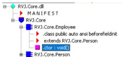
Figure 4-6. The RVJ.Core.Business.Employee::.ctor() is declared/defined with this special name in MSIL for a default instance constructor
