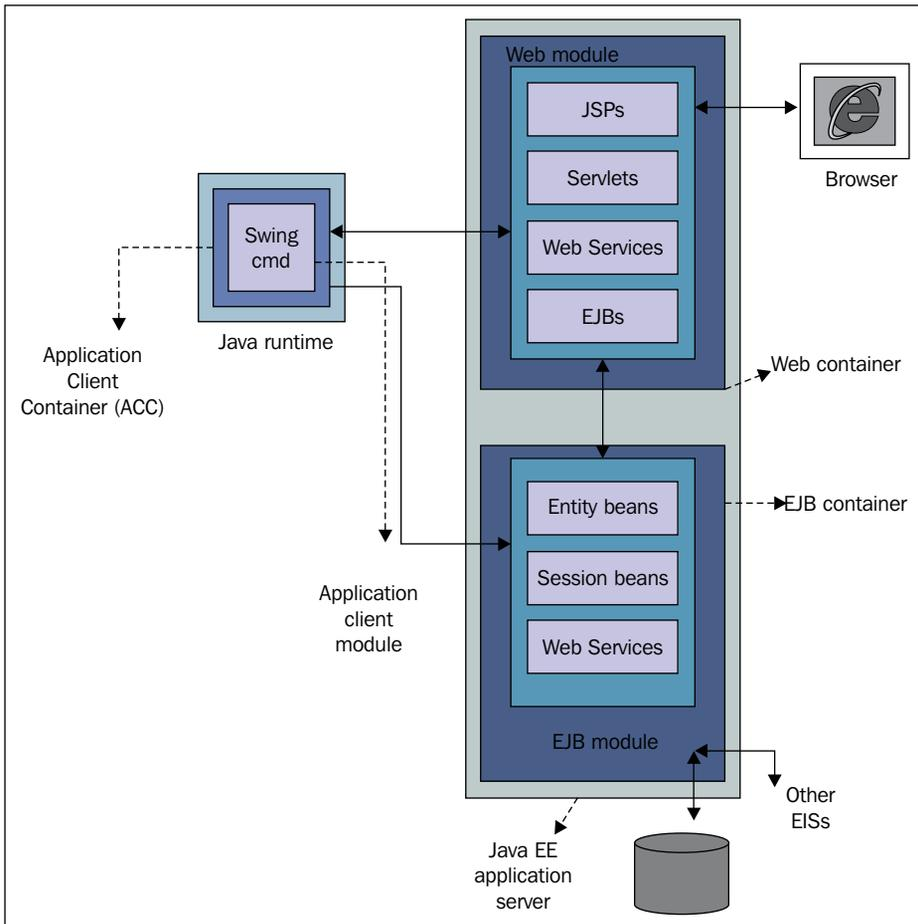
The previous figure assumes that no security measure is applied on user interaction with application or the interactions between different application modules. Each of these modules can be deployed independently or one or more of them can be included in a larger logical bundle named **Enterprise Application Archive (EAR)** and deployed together into the application server. Application server will decompose the archive and deploy each module into its designated container.
