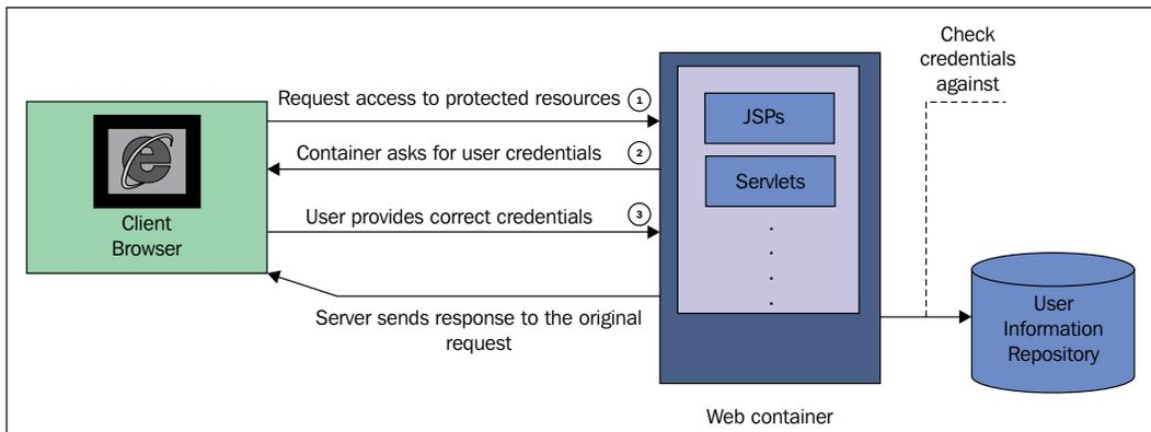
The previous figure illustrates steps the clients need to go through when they try to access some restricted resources. The Web container protects the Web module content by checking the requested URLs and decides whether it should send back the corresponding response or prevent the request going through the normal procedure until it ensures that the entity which requested the resource is permitted to access that specific resource.
