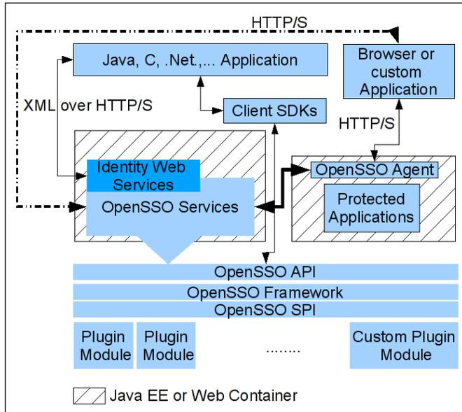
As you can see in the figure, all of the lower-level blocks are running inside an application server or a Servlet container. You can see that multiple types of client applications may interact with the OpenSSO server. These applications can be one of the following types:
