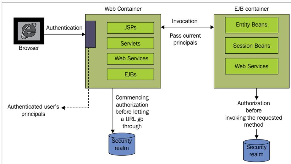
Whenever the Web container needs to invoke some methods from an EJB module in the EJB container it sends the authenticated user's principal to the EJB container, which goes through authorization to see whether the current user has the permission to invoke the method or not.
