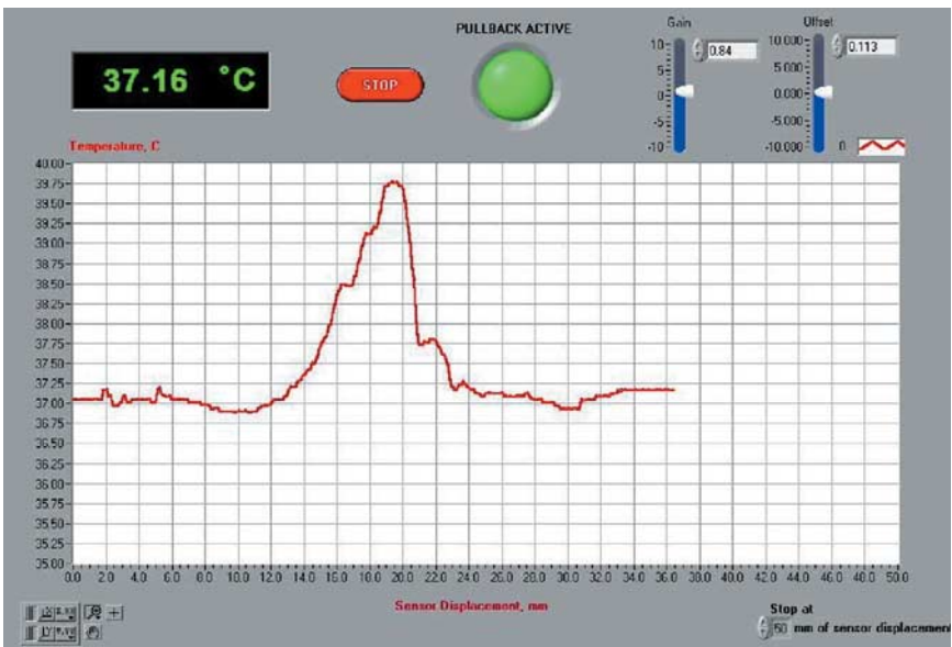
Figure 19.2 Temperature heterogeneity: temperature data from the thermocoil guidewire tip during rotational pullback through a fluid-filled plastic tube with a short external heat source adjacent to one aspect.
