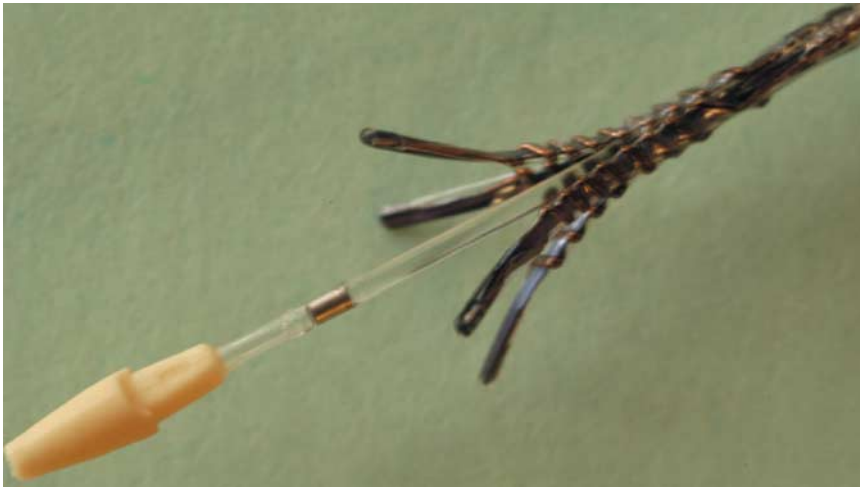
Figure 20.2 Close-up photograph of a catheter illustrating the four expanded thermistors.
