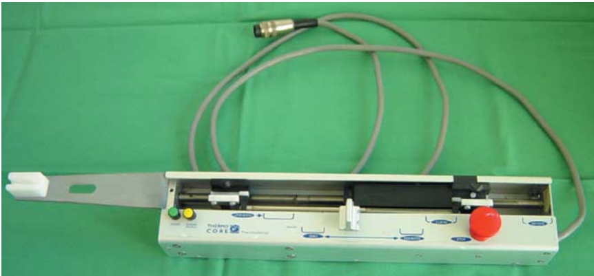
Figure 20.4 The pullback system is placed on the operating table during the procedure, covered by a sterile sheath.
