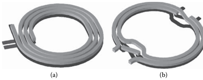
Figure 4.1 (a) Asymmetric and (b) symmetric stacked transformers.
