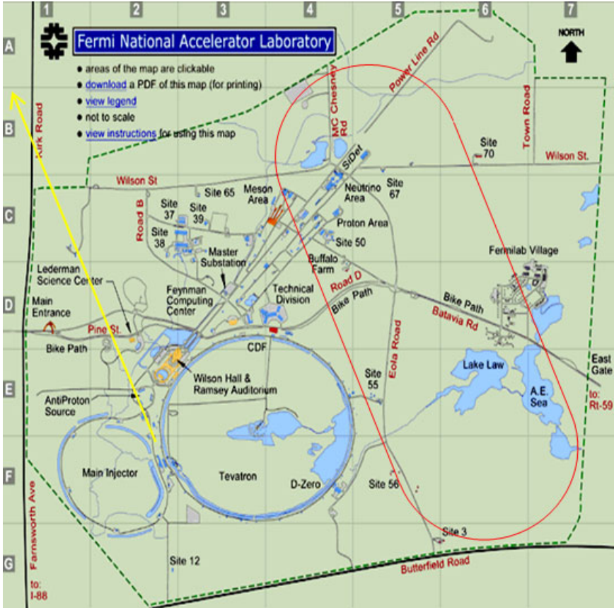
Fig. 2.22 A beta beam decay ring with a magnetic rigidity of 1500 Tm and a gamma of 300 would fit on the present Fermi laboratory site. Illustration courtesy of Andreas Jansson from FNAL.
