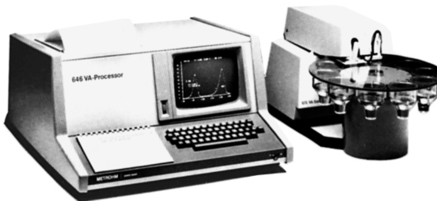
FIGURE 4-4 Microprocessor-controlled voltammetric analyzer, in connection with an autosampler. (Courtesy of Metrohm Inc.)
