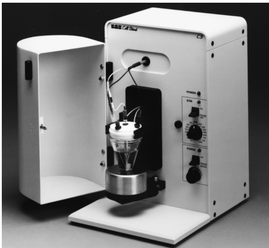
FIGURE 4-2 A complete cell stand. (Courtesy of BAS Inc.)
