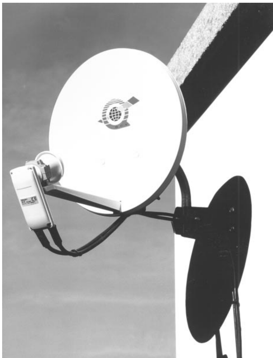
Figure 8.7 A 12-GHz MVDS receiver with 35-cm dish antenna and LNB (installed in Qatar). (Courtesy of GEC-Marconi.)
