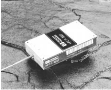
Figure 3.5 50–622-Mbps (STM-4) transmitter for single-mode fiber. (Courtesy of Hewlett-Packard.)
