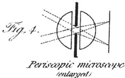
Fig. 6.5. Wollaston's Periscopic Microscope Lens, 1812.
