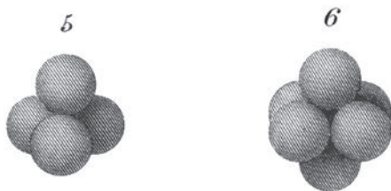
Fig. 9.4. Construction of a Tetrahedron and an Octohedron from Spheres.
