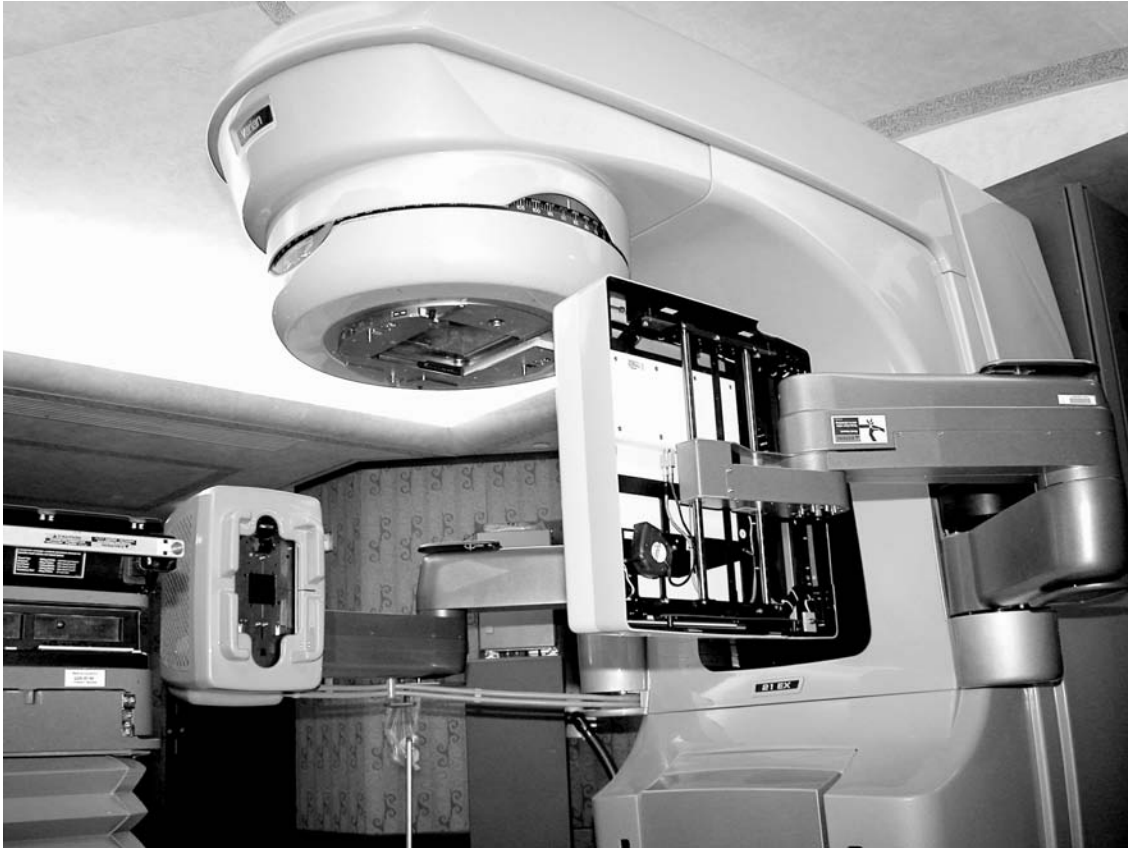
Figure 16.2 Varian kV Imaging system (OBI). The kV source, kV detector, and MV detector are all mounted on robotic arms.
