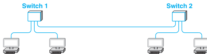
Figure 25.4 Four hosts connected by two switches.
