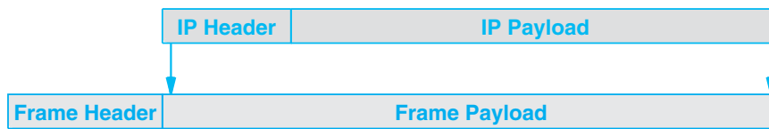
Figure 22.7 Illustration of an IP datagram encapsulated in a frame.
