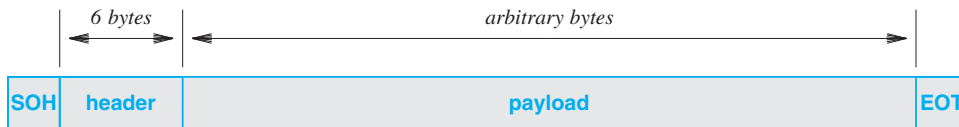
Figure 13.11 An example frame format that uses SOH and EOT characters to delineate a frame.
