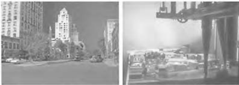
1.6 The three-dimensional model as a visualization environment: (right) a view of an urban streetscape (with manual editing); (far right) the gantry system which carried the camera along defined paths
