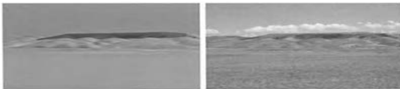
8.5 Site C as seen from KOP 13 showing the use of three-dimensional modelling as a guide for image-based simulation: (left) three-dimensional model of site from 3DstudioViz; (right) photograph of the site with three-dimensional model overlay
