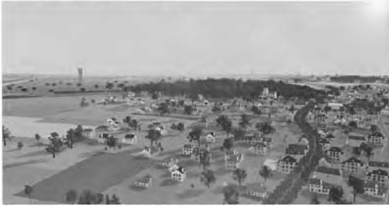
2.9 The distinction between geospecific and geotypical textures and objects: (left) geospecific ground texture and geotypical trees; (below) geotypical ground textures and housing
