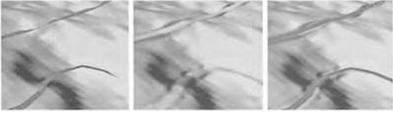
3.5 Carving a terrain to match a road surface: (left) naïve drape with intersection problems; (middle) terrain carved to match road surface; (right) a drape with better results
