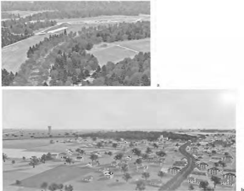
2.9 The distinction between geospecific and geotypical textures and objects: (a) geospecific ground texture and geotypical trees; (b) geotypical ground textures and housing (images reproduced in the colour plate section)
