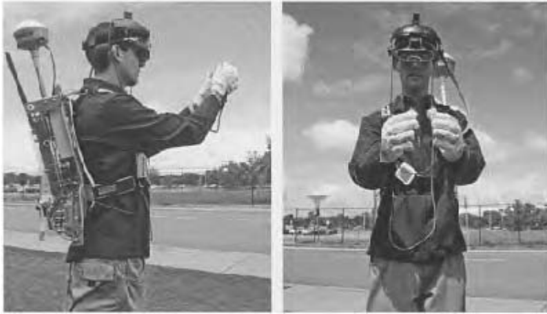
10.5 Tinmith-Endeavour outdoor augmented reality mobile computing system
