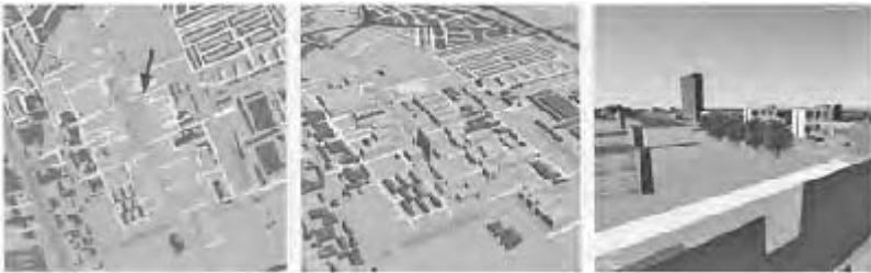
2.10 The three views of GIS data as defined by Verbree et al. (1999): (left) plan view; (middle) model view; (right) world view
