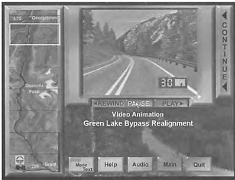
5.5 Sample frame from the Guanella Pass Proposed Road Improvements Project CD ROM, showing a drive-through video-animation in a user-selected driving sequence of the proposed highway improvements (image reproduced in the colour plate section)
