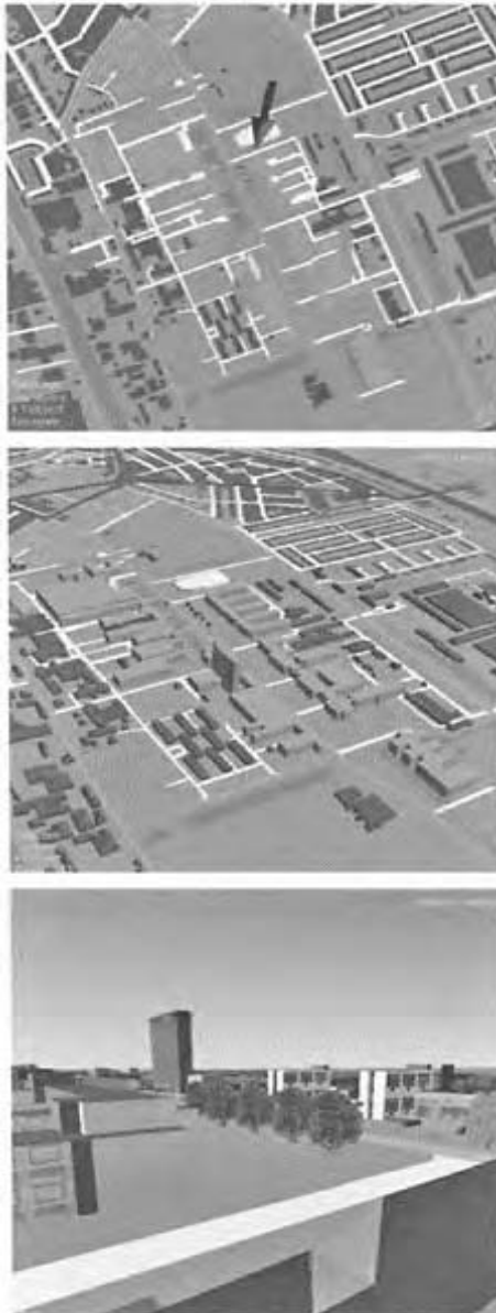
2.10 The three views of GIS data as defined by Verbree et al. (1999): (top) plan view; (middle) model view; (bottom) world view (images reproduced in the colour plate section)
