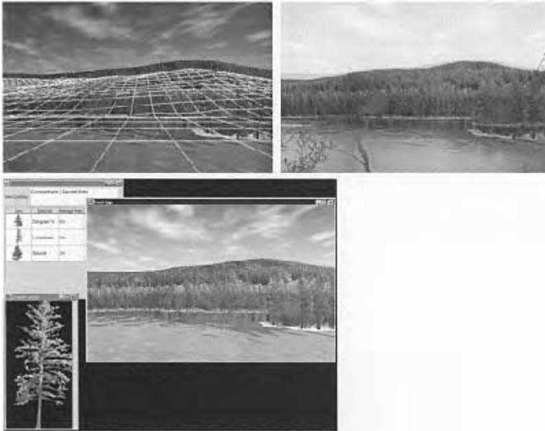
5.6 Making visualizations transparent—a simple Java application interface designed to display simultaneously both the modelled image and the underlying data: (top left) three-dimensional forest canopy wire-frame model; (top right) existing site photograph; (left) billboarded tree templates
