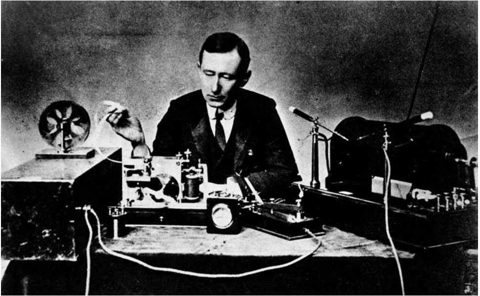
Italian physicist Guglielmo Marconi, who claimed he invented radio, reads signals on a tape recorder, left, with a 10-inch spark coil used for ship-to-shore radio tests in this 1901 photo. [AP Photo]
