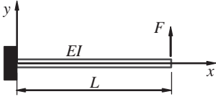
Figure 1.6. A cantilever beam.
