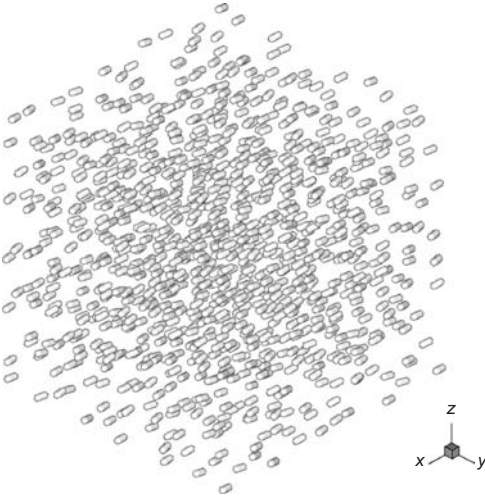
Figure 6.6. A BEM model of 1000 capsulelike scatterers with a total of 200,000 elements.
