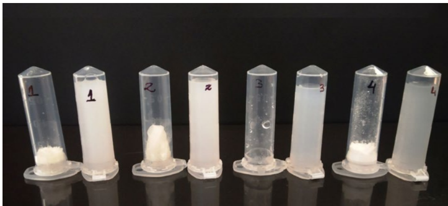
Figure 2.1. Freeze-dried emulsions using different cryo- or lyo-protectants and reconstitution of freeze-dried powder into nanosized emulsion. (See color insert.)
