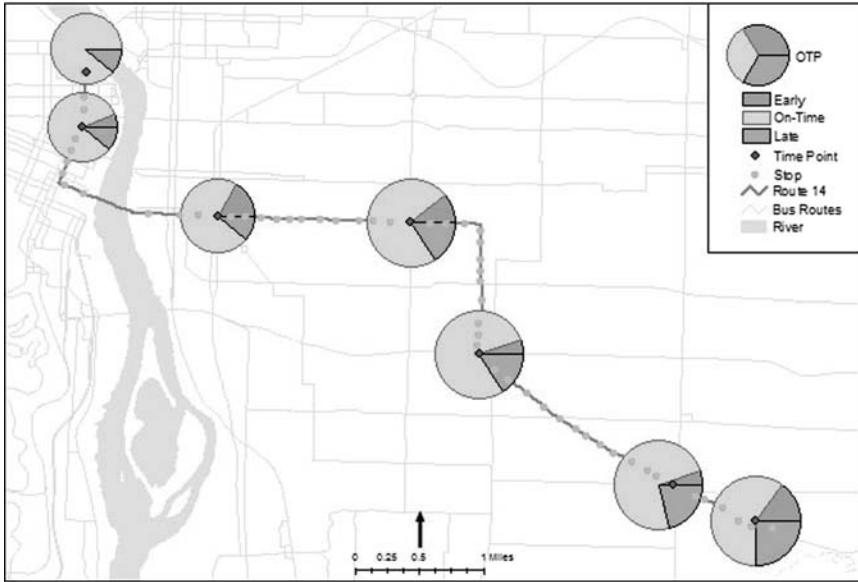
Figure 27.5: On-time performance visualization by stop location. Source: Kimpel (2007, p. 20), reprinted with permission.
