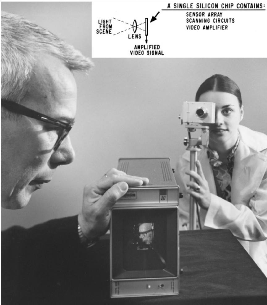
Technician Lynn Roberts captures Winthrop Pike at RCA's David Sarnoff Research Center with an early CCD camera in March 1972, two years after AT&T announced the technology. The use of photosensitive solid-state elements eliminated the bulk and delicacy of vacuum tubes and their glass envelopes. David Sarnoff Library
