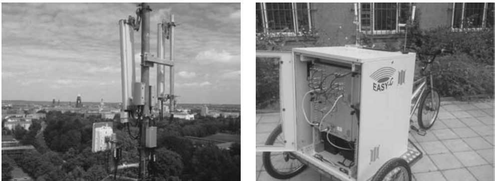
Figure 5.16 Dresden's Easy-C platform consists of cooperating BSs (left) and nomadic MSs on the ground (right) [558]
