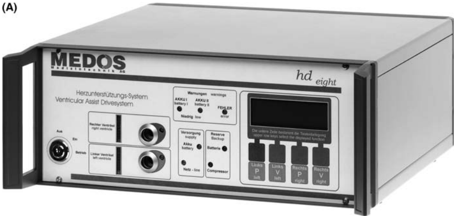
Figure 4 (A) SynCardia MEDOS HD8™ Mobile Driver. (B) Berlin Heart EXCOR™ Portable Driver. (Continued)
