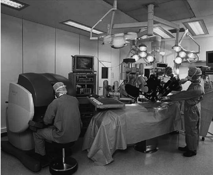
Figure 1 Components of the da Vinci ® Surgical System. This system consists of a surgeon “master” console ( left ), video cart ( center ), and “slave” tableside robot with two or three instrument arms and a stereoscopic endoscope ( right ). Source: Photo courtesy of Intuitive Surgical, Sunnyvale, California, U.S.A.
