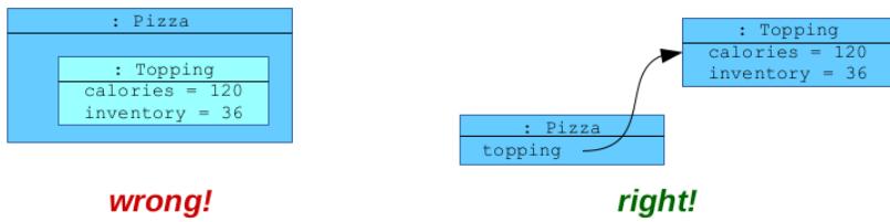
Figure 6.4: The wrong, and right, way to visualize a “has-a” association in Java.
