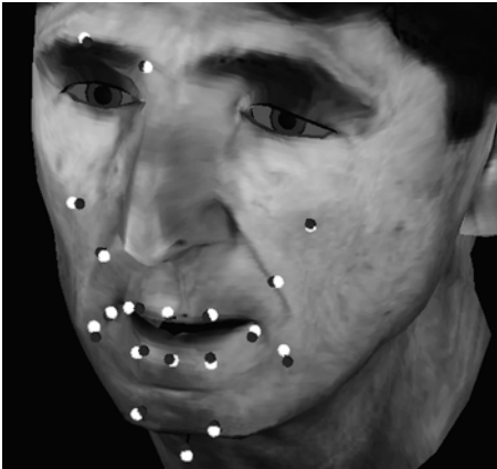
Figure 12.15 Illustrates placement of the points for the new model of WM, which corresponds to Baldi's wireframe morphed into the shape of DWM. These dark points are placed 3mm (4mm for the chin point) off the synthetic surface and the placements of the corresponding measured OPTOTRAK points are given in white.
