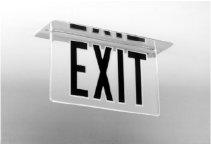
Figure 9-4. Edge-lit exit signs are clear panels with the light source(s) mounted across the top edge. As light passes down through the panel, the letters are illuminated. Courtesy: Lithonia Lighting.
