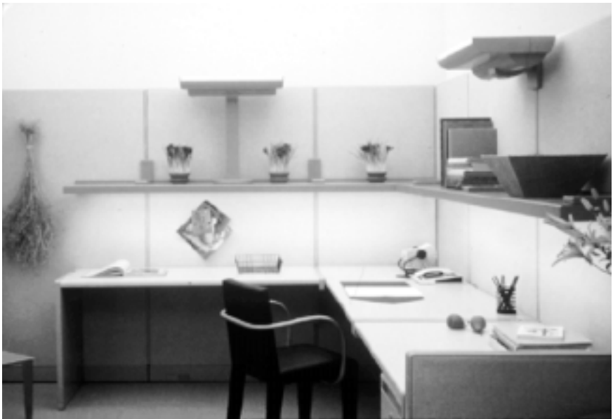
Figure 14-5. Furniture-mounted uplighting and task lighting work together to provide high-quality, energy-efficient illumination. Courtesy: Peerless Lighting Corporation. Photo by John Sutton.
