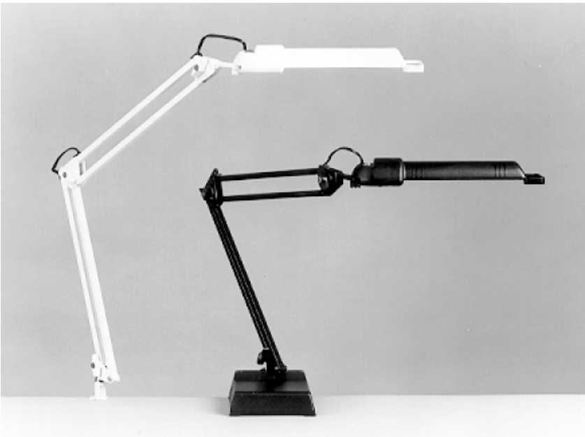
Figure 5-9. Compact fluorescent task lights give occupants control over their illumination. These task lights feature articulating arms that enable the user to position the task light for optimal task visibility. Courtesy: Dazor Manufacturing Corporation.
