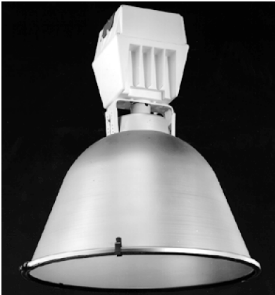
Figure 16-4. When used in dirty environments, HID luminaires should be enclosed and gasketed to keep dirt off the lamps and reflector surfaces. And use enclosed HID luminaires where metal halide lamps are not rated for open luminaire operation. Courtesy: Thomas Lighting.
