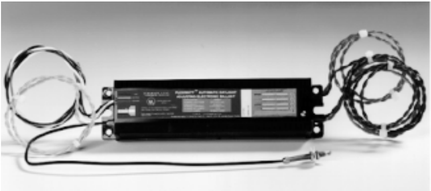
Figure 12-3. Retrofit daylight-dimming installations can be affordable when tandem-wiring 4-lamp dimming electronic ballasts and using integrated light sensors. These systems can be manually adjusted to provide location-specific light levels (tuning). Courtesy: Flexiwatt, LCC.
