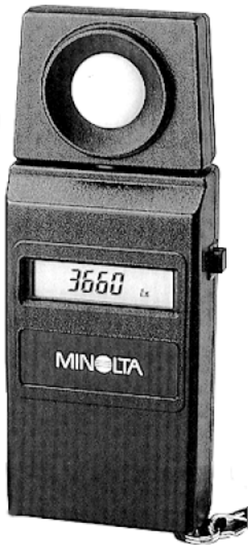
Figure 18-4. Illuminance meters can measure light levels in footcandles (fc) or lux (lx). This meter can be reconfigured to read either value. Courtesy: Minolta.
