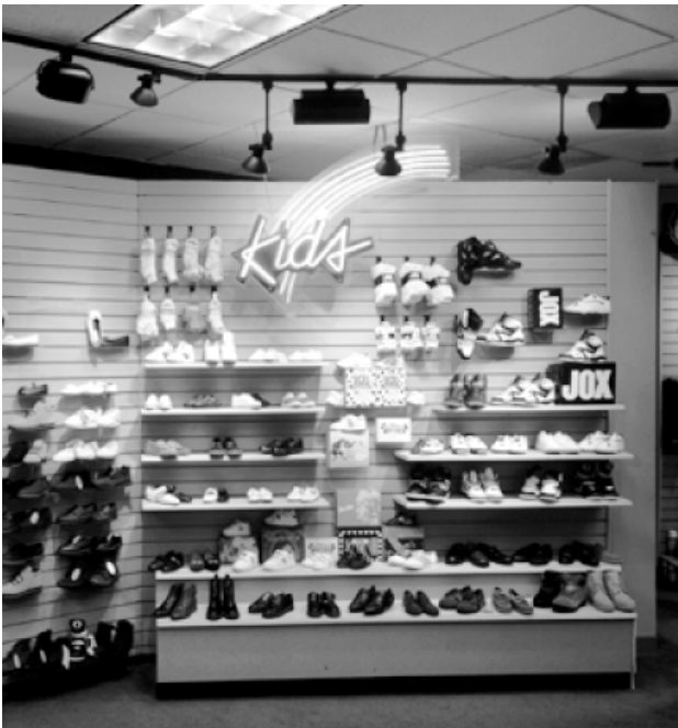
Figure 15-2. Medium-activity stores typically combine low-glare fluorescent ambient lighting with brightly illuminated feature displays. Courtesy: Lightolier.
