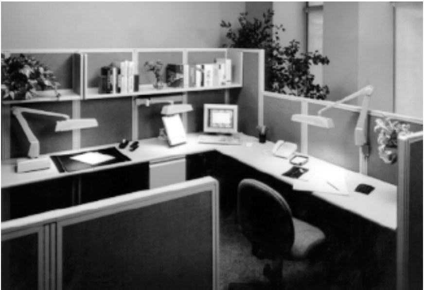
Figure 4-17. Compact fluorescent task lights can be repositioned by the user to minimize reflected glare and to illuminate specific task areas. Courtesy: Dazor Manufacturing Corporation.
