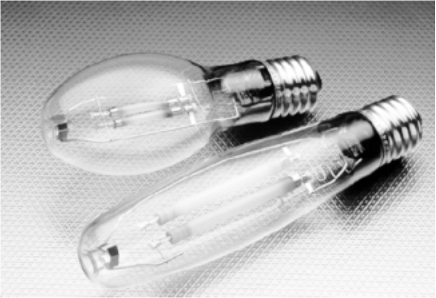
Figure 8-1. “Instant-restrike” high-pressure sodium lamps use two arc tubes. The “standby” tube is ready for restriking in the event of a short power interruption. Courtesy: GE Lighting, Cleveland.
