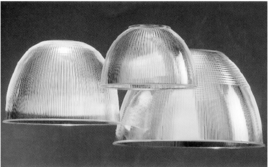
Figure 8-4. Existing HID luminaires can be retrofitted with clear reflectors which direct most of the light down to the work surfaces. Some of the light is refracted toward the ceiling and walls, providing diffuse reflected light for improving illuminance on vertical surfaces. This product allows flexible lamp positioning which offers a range of spacing criteria and uplighting percentages. Courtesy: Lexalite International.
