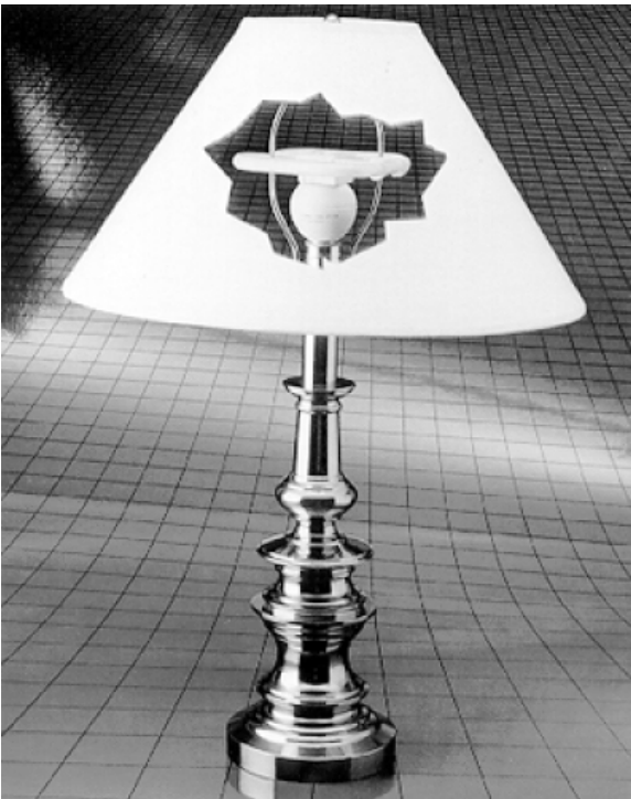
Figure 5-10. Table lamps can be retrofit with either 2-D or spiral-type compact fluorescent lamps, using electronic ballast adapters for instant starting, light weight and improved efficacy. These lamps provide high color rendering (82-86 CRI) and uniform lighting. Courtesy: Alta Illumination Co.
