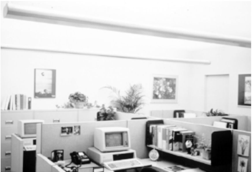
Figure 4-15. Indirect luminaires can enlarge the perceived size of the space by illuminating the ceilings and upper walls. Courtesy: Peerless Lighting Corporation. Photograph by Richard Sexton.
