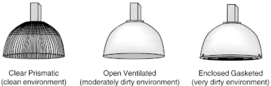
Figure 7-8. The selection of high-bay HID luminaires is driven by the type of dirt conditions in the space. In addition, some metal halide lamps must be used in enclosed fixtures; others are rated for use in open fixtures. Courtesy: EPA Green Lights.
