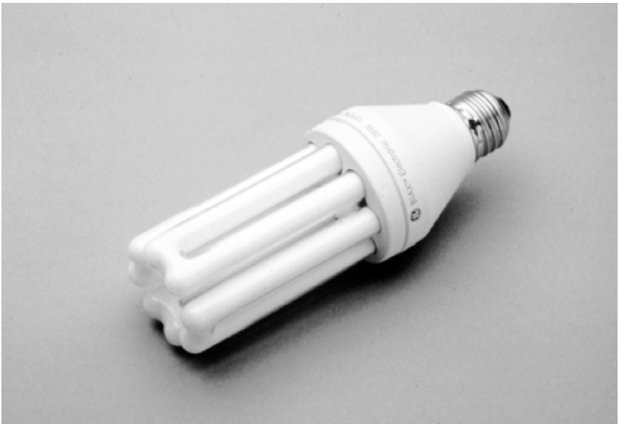
Figure 6-3. This 28W lamp contains four twin tubes and is designed to be used in applications normally served by 100W general-service incandescents. Courtesy: GE Lighting, Cleveland.
