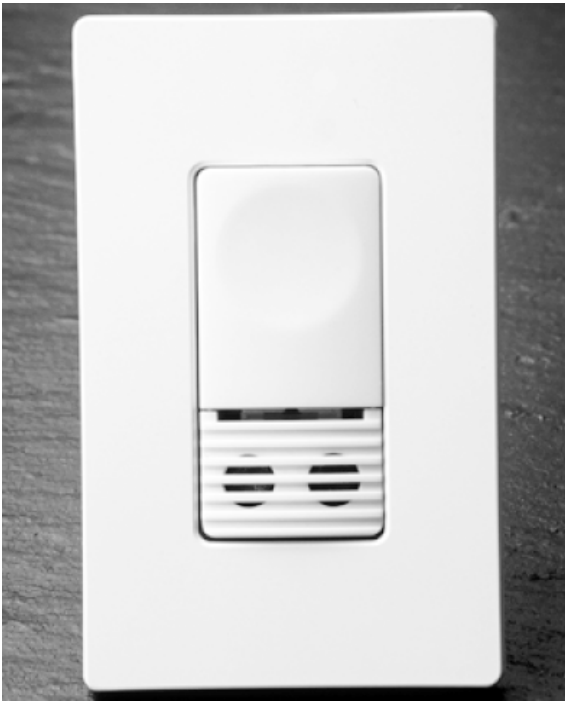
Figure 11-4. Switch-mounted ultrasonic sensor with manual-on option. This sensor can be configured for automatic-on operation if desired. Courtesy: Novitas, Inc.
