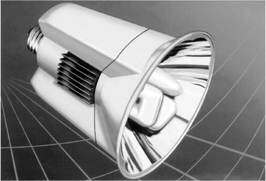
Figure 6-2. With advanced reflector designs, manufacturers are producing compact fluorescent reflector lamps with improved center beam candlepower, suitable for higher mounting heights (over 15 ft.). Courtesy: ProLight.
