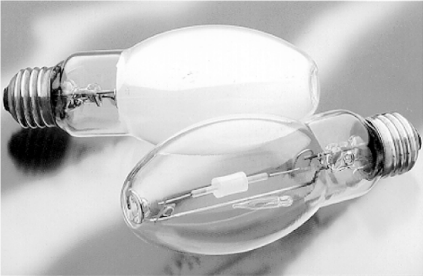
Figure 5-6. New low-wattage metal halide lamps with ceramic arc tubes replace incandescent lighting in non-dimming applications. Used with a specially designed electronic ballast, the system provides high efficacy and excellent color rendering. The small size of the arc tube allows for tight beam control in directional lighting applications. Courtesy: Philips Lighting Company.
