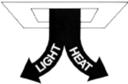
Figure 18-1. All of the energy that is consumed to produce light is eventually converted to heat. Therefore, reductions in lighting energy use will produce reductions in air conditioning costs. These savings can be much higher than any heating “penalties” resulting from a lighting upgrade, particularly in the southern latitudes. Courtesy: National Lighting Bureau.
