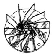
The impeller fan of a vacuum, the part that creates the suction
