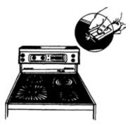
The manufacturer may recommend using a razor blade for hardened spills—follow the directions carefully! Never use green scrub pads or pads with metal fibers such as steel wool. And keep abrasive cleaners, oven cleaner, bleach, and rust remover well away.
