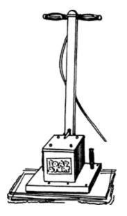
A floor machine of the type used for bonneting.
