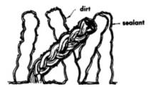
SEALED CONCRETE (nonporous) Has a smooth, easily cleanable surface, and stains and spills can't penetrate.
