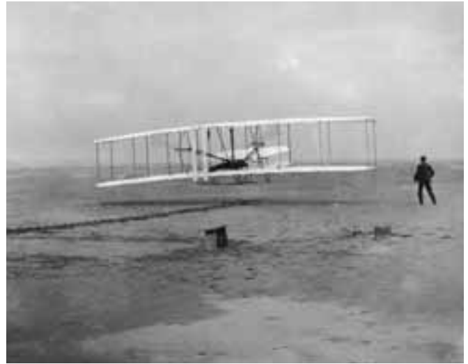
This historic photograph is of the Wright Brothers' first successful powered flight, December 17, 1903, 10:35 A.M. Orville is in the plane, and Wilbur is running alongside. The starting rail is visible on the ground. ( Library of Congress, Prints and Photographs Division, LC-USZ62-6166A )
