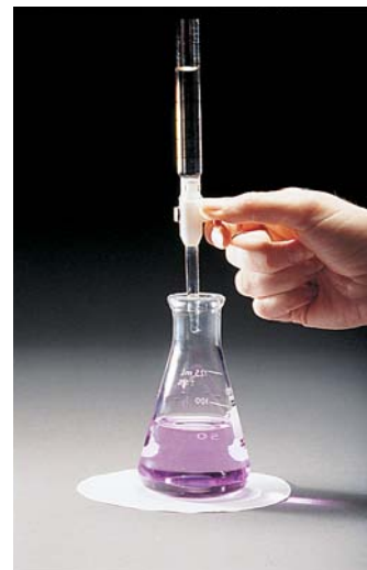
Figure 3. The experimental setup for an acid-base titration.
