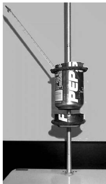
Figure 2. Set up of a soda can calorimeter
