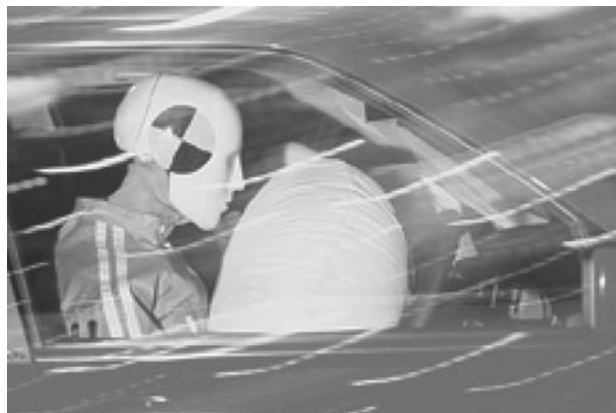
Figure 1. Deployment of an automobile airbag on a test dummy.
