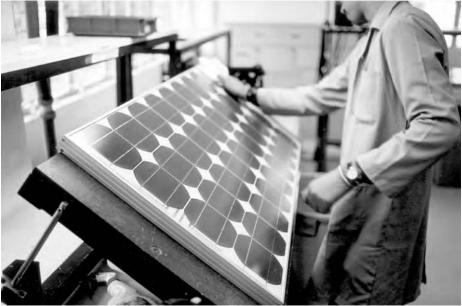
Figure 1.9 A solar PV module coming off the manufacturing line
