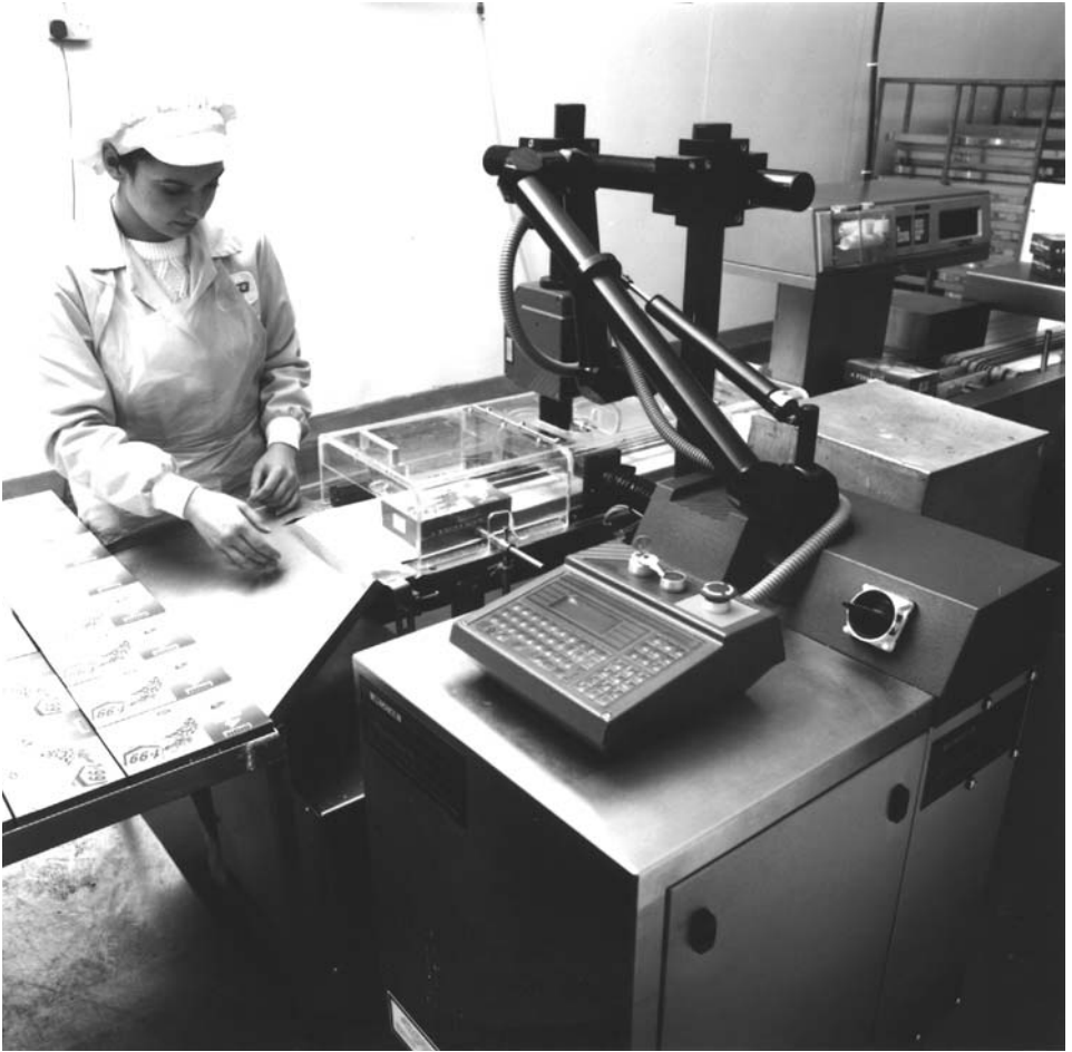
Fig. 24.11 Laser coding: (a) (above) operator interface and coding laser on a production line; (b) (overleaf) date and production codes positioned on a carton. (Courtesy of Lumonics Ltd.)
