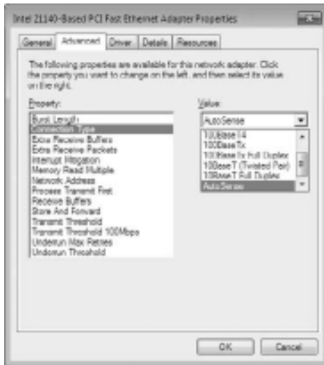
Figure 9.6: You can click the Advanced tab to see additional properties specific to the device.
