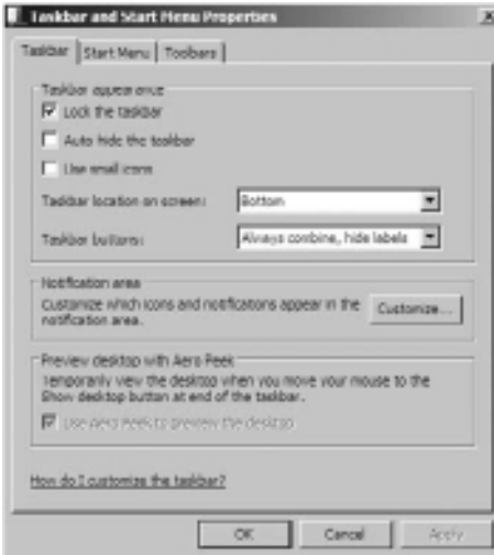
Figure 4.7: The Taskbar tab of the Taskbar And Start Menu Properties dialog box
