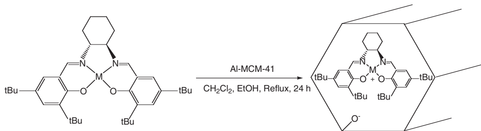
Scheme 2.1.6.4 Method for the impregnation of metal-Jacobsen complexes into Al-MCM-41.
