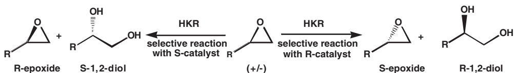
Scheme 2.1.6.5 Hydrolytic kinetic resolution (HKR) of terminal epoxides.
