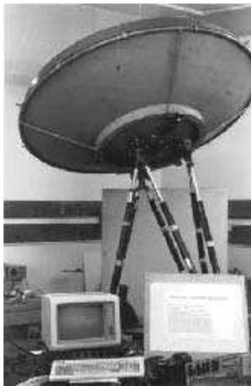
Figure 2.7. Use of a parallel robot to position antennae. Notice the small size of the actuators in comparison to the parabola
