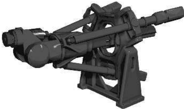
Figure 2.19. The Neumann prototype. A rod of variable length, mounted on a joint, connects the end-effector to the base (according to Neumann [NEU 88]. Three linear actuators enable motion of the end-effector
