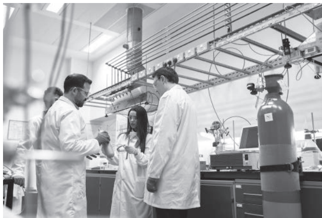
Figure 13.1 Safety in a research laboratory. Safety was partly designed in at the start. For example, tubes carrying different gases are clearly marked and RCDs are in place to protect from electric shock. However, administrative controls are also needed by users—for example, maintaining accurate records of chemicals in use, ensuring that people who use the laboratory know how to handle the chemicals safely, and ensuring that PPE is worn.
