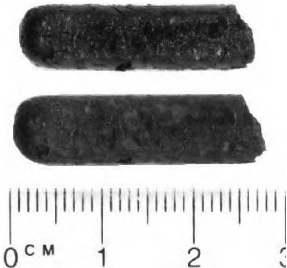
Figure 2.13. Photograph of the shaped magnetic ceramics obtained from crosslinked poly(ferrocenylsilane) precursor materials. Reproduced with permission from [96].
