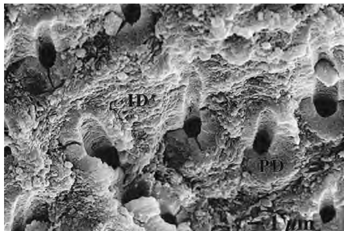
Figure 1.8. Scanning electron micrograph of a fracture surface through crown dentin of a human tooth. Various tubules are viewed in cross section. The dense envelope around the tubules is composed of peritubular dentin (PT). Intertubular dentin (ID) is located in the intervening spaces.
