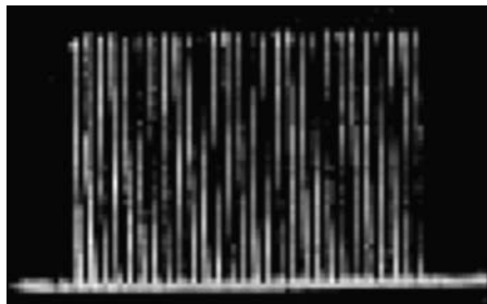
Figure 13.4 Spectrum of the radiated signal produced by an FHSS technique
