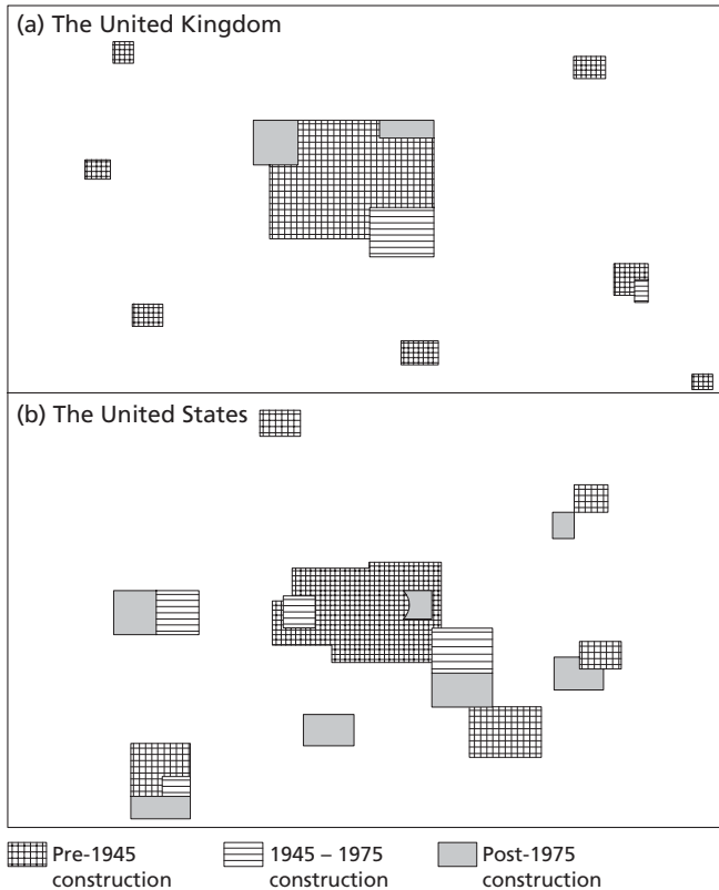
Figure 4.3 Contrasting patterns of urban development: the United Kingdom and the United States. In the United Kingdom cities have tended to be contained by strict planning legislation which has mandated a so-called greenbelt around the city. Within the greenbelt it is very difficult to obtain the necessary planning permission. Expansion to meet the city's needs for additional housing typically occurs either on the edge of the city, as demonstrated in the schematic figure, through densification of already developed areas and, at one time, through the construction of high rise, publicly owned, blocks of flats. In surrounding villages (indicated by places that have clearly not grown since 1945) development is limited by the fact that they are "in the greenbelt." What development occurs is largely what is called "infill" or through the conversion of existing structures from lower-income to higher-income use. The typical pattern in the US is very different. There is no cordon sanitaire in the form of a greenbelt, and in consequence housing densities can be much lower as the city expands at its edge. Nearby villages also add new residential development until it joins up the developing edge of the nearby city into a low-density pattern that has become known as "urban sprawl."
