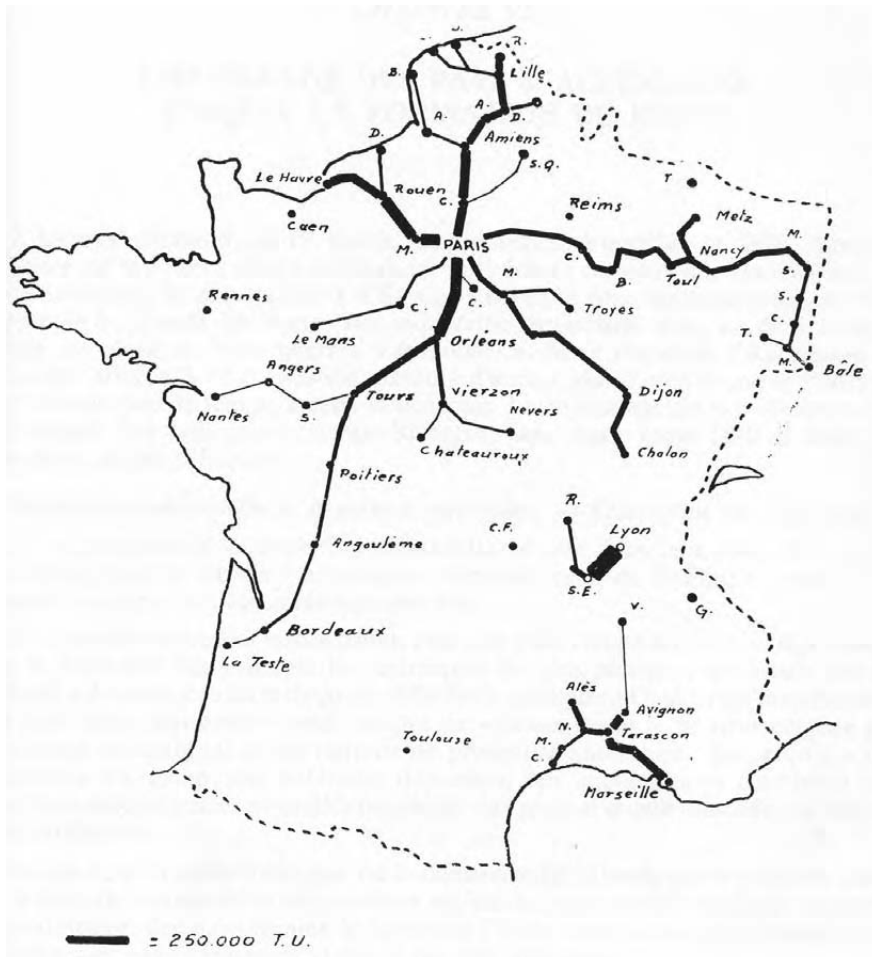
Figure 9. Merchandise traffic by rail in France. Annual throughput by line section (in effective thousands of tons) in 1854. Extract from Renouard, Les transports des marchandises depuis 1850 , Armand Colin
