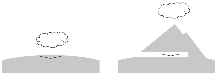
Fig 9.1 Left: The gravitational attraction of a dense cloud can move the mirrors in an interferometer on the ground. Right: For an interferometer such as KAGRA deep under a mountain, the cloud is farther away, reducing its gravitational effects.
