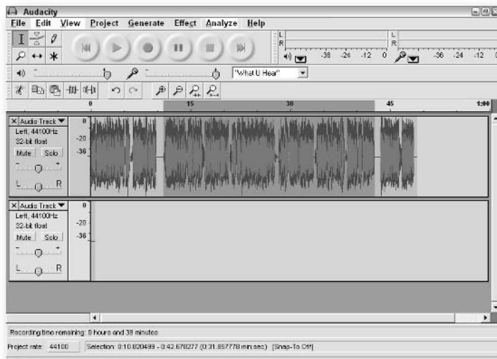
FIGURE 9-14: Audio from bottom track spliced into top track.
