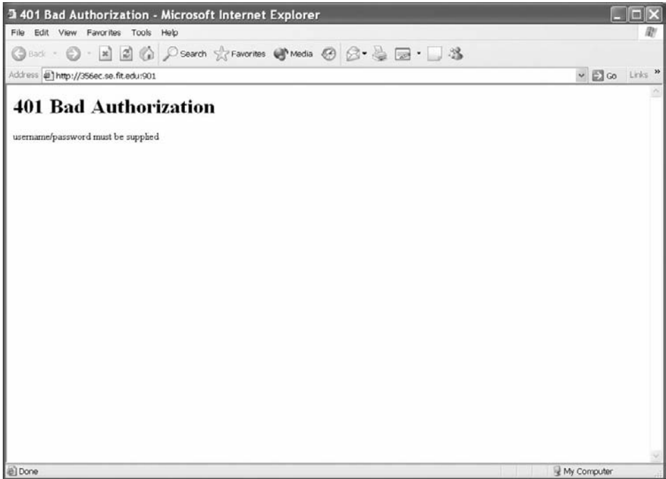
FIGURE 17.4 “Bad Authorization” result from invalid username.
