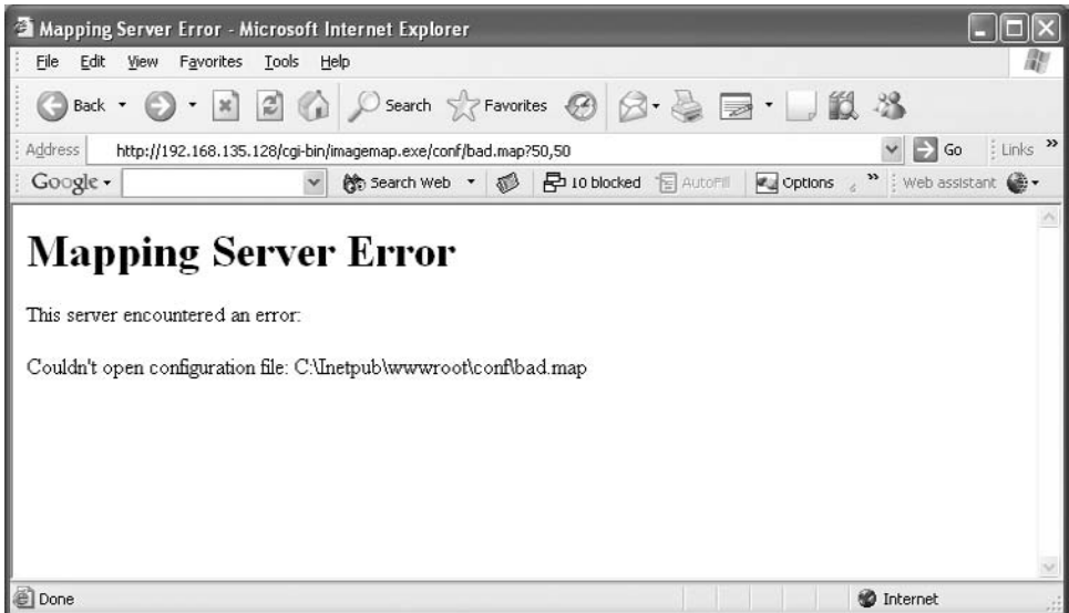
FIGURE 17.6 Error message exposing information about the organization of the filesystem on the server.
