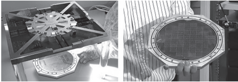
Figure 18.7 Silicon wafer and aluminium back panel, hexagon silicon wafer (Meier, 2012). The simulations for the chips were run on JUGENE computers and communication between on-wafer neurons was established (Meier, 2012).
