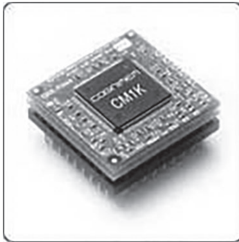
Figure 18.6 CM1K chip (General Vision, 2018).
