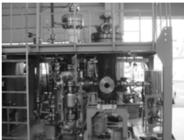
Figure 5.3. HyPr-Ring pilot-scale demonstration unit with 3.5-kg/h coal process rate. With permission from Dr. Shiyong Lin of Japan Coal Energy Center; photo presented at the 3rd International Workshop on In Situ \text{CO}_2 Removal, ISCR, 2007.
