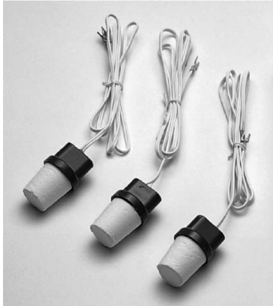
Figure 2.13 Gypsum blocks of Soilmoisture Equipment Corporation. Courtesy Soilmoisture Equipment Corp
