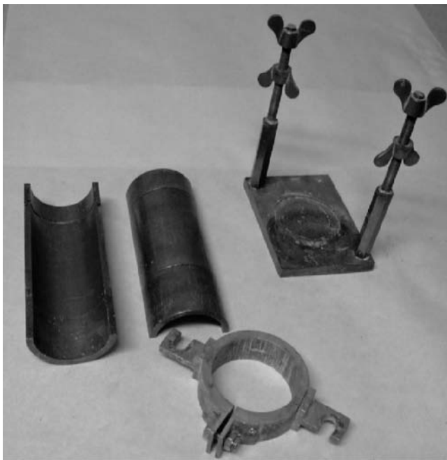
Figure 3.2 Compaction mould (50 mm diameter and 150 mm height).
