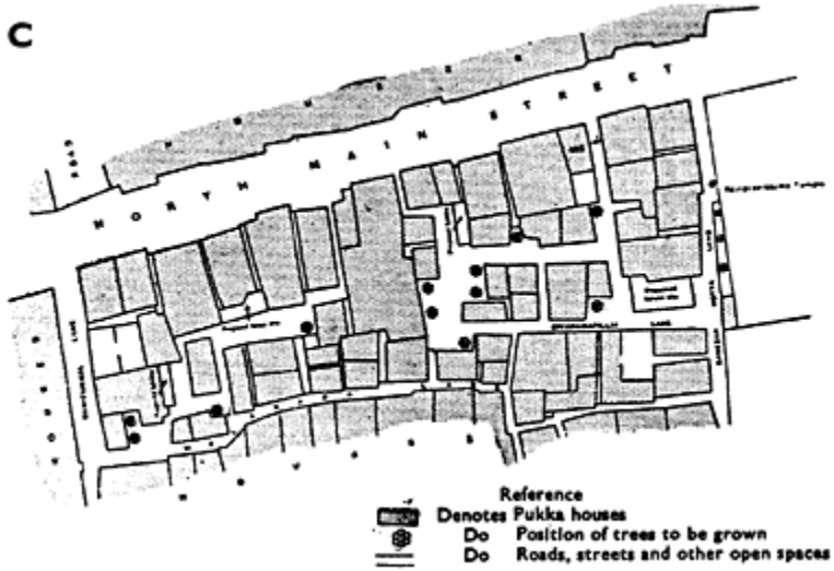
Plan C shows 'the congested area as it would appear after the application of conservative surgery. Cost about Rs 5,000'. The old street pattern has been kept, open spaces created and trees planted. (Source: Tyrwhitt, 1947)
