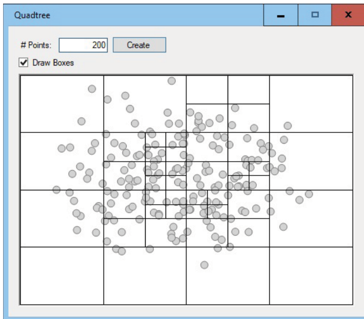
Figure 10.25: Each box shows a quadtree node's area.
