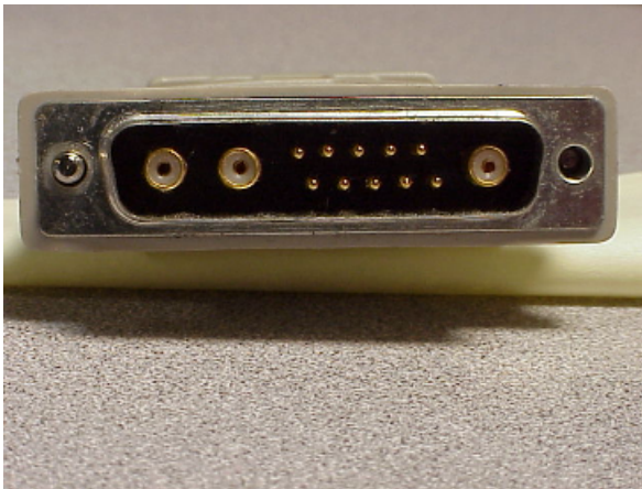
Figure 9-9 The 13W3 connector. This type, common in the workstation market, also uses a “D”-shaped shell, but has three true coaxial connections for the RGB video signals, in addition to 10 general-purpose pins. Unfortunately, the pin assignments for this connector were never formally standardized. Used by permission of Don Chambers/Total Technologies.
