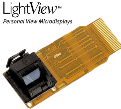
Figure 4-17 An LCOS microdisplay product with an integral light source, for near-eye use. The LCOS device itself is mounted on the flexible substrate, underneath the black plastic structure that carries LEDs (on the upper left of the housing, as seen here) and a curved film which acts as a polarizing beamsplitter. (Picture courtesy of Displaytech, Inc.; used by permission.)
