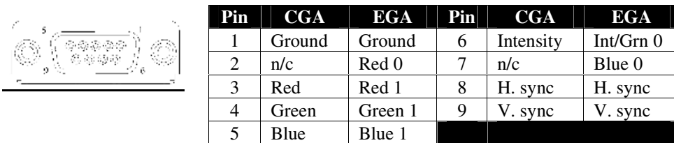
Figure 9-3 The revised pinout of the 9-pin connector for the Color Graphics Adapter (CGA) and Enhanced Graphics Adapter (EGA) products.
