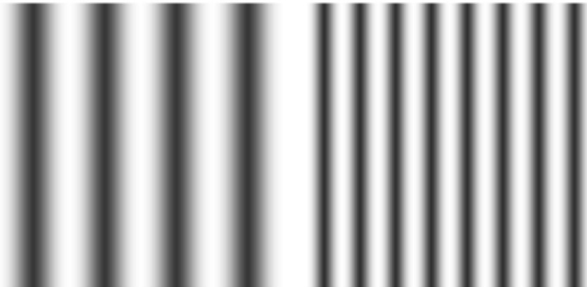
Figure 2-5 Two patterns of different spatial frequencies. The pattern on the right has a frequency, along the horizontal direction, roughly twice that of the pattern on the left. (Both represent sinusoidal variations in luminance.) It is common to express both display resolution and visual acuity in terms of the number of cycles that can be resolved per unit distance or per unit of visual angle.
