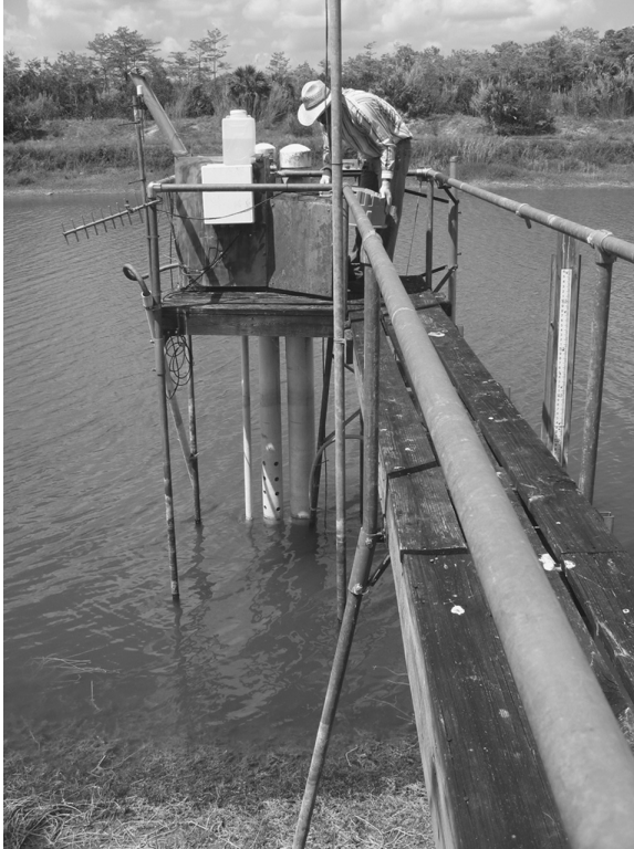
FIGURE 14.2 A PVC pipe with holes at the bottom to let water run through, for Hydrolab installation on a platform at a canal sampling site.
