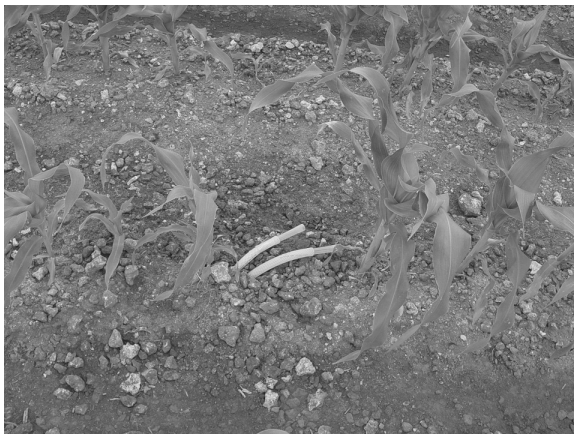
FIGURE 7.7 After installing the lysimeter, the two flexible tubes are left protruding from the ground. Water collected in the lysimeter is removed using the two tubes: one tube serves as an air vent while the other is connected to a peristaltic pump. It is important to secure (but not to an airtight seal) the exposed tube ends to ensure that dirt, debris, or insects do not enter the tubing. If the air vent tube is airtight, no leachate will be collected in the lysimeter irrespective of the rainfall/irrigation water applied.
