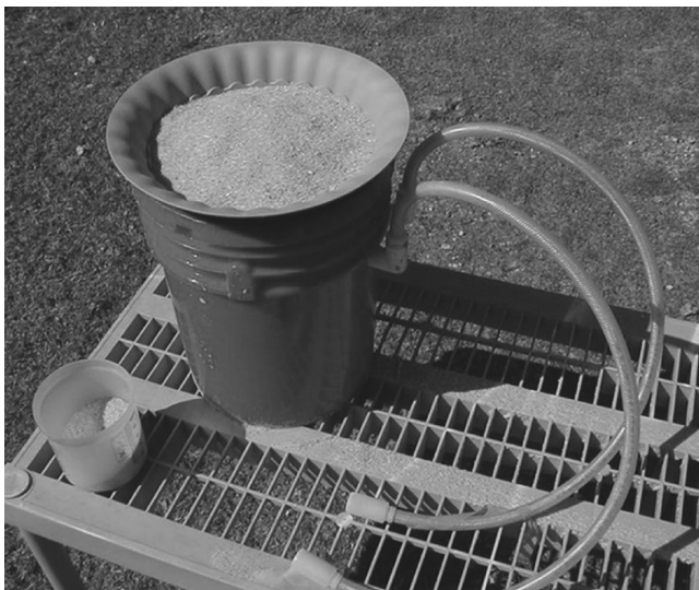
FIGURE 7.4 Lysimeter with sand placed in collecting plate and flexible tubing attached for sample collection.
