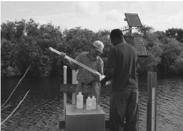
FIGURE 14.4 Bailer used for surface water grab samples at canal sampling site.
