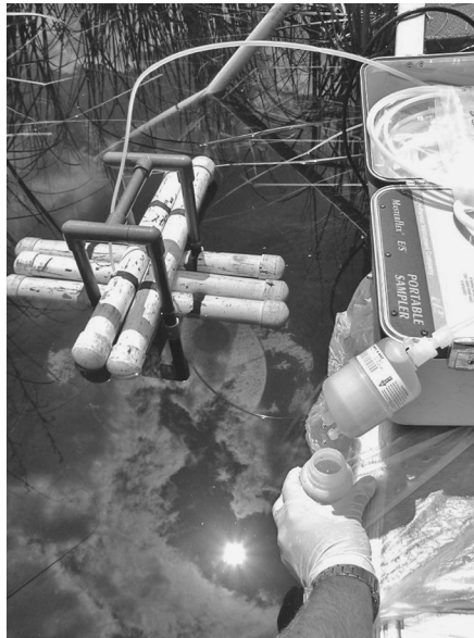
FIGURE 7.14 Deploying the modified sipper at the sampling site with a set of five, equally distributed 12 kg weights laid across the handle cross-bars.
