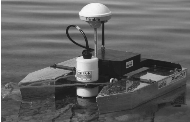
FIGURE 14.3 The SonTek RiverCAT for canal profile measurement.
