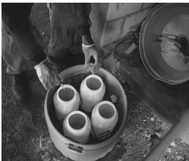
FIGURE 14.5 Containers in the auto-sampler of ISCO 6712.
