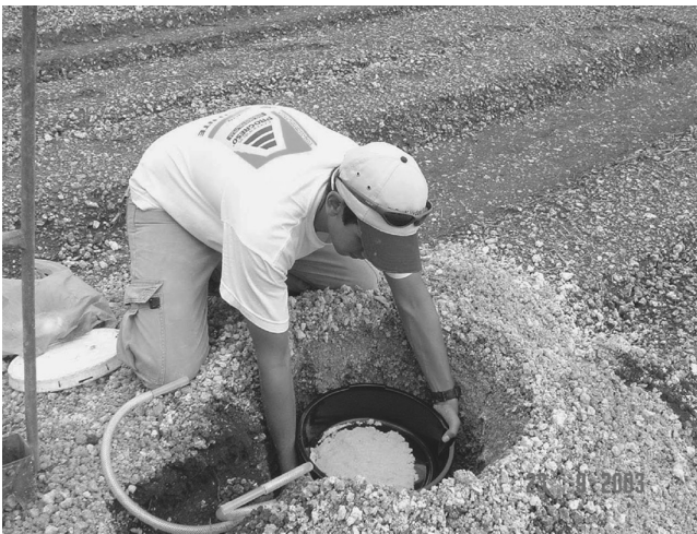
FIGURE 7.6 Installing a bucket lysimeter.
