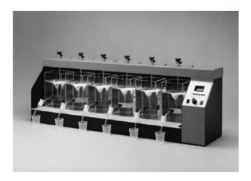
FIGURE 5-3. PB-700 Series Six-Paddle Standard JarTester. (Phipps & Bird.)
