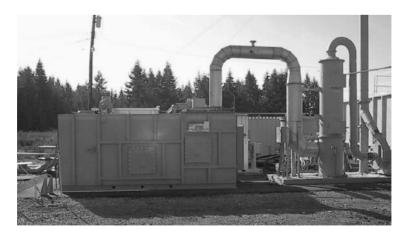
**FIGURE 6-13.** Catalytic oxidizer with integral scrubber. (Photograph provided by Anguil Environmental Systems, Inc.)
