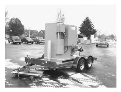
**FIGURE 6-11.** Small electric catalytic oxidizer. (Photograph provided by Catalytic Combustion Corporation.)
