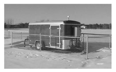
FIGURE 7-5. Trailer-mounted mobile soil vapor-extraction unit.
