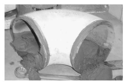
FIGURE 7-3. Silt material collected in the system piping.
