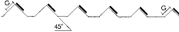
c. Increasing height, front (smallest) tooth identical to any tooth in b, subsequent teeth have equal areas of PV and glazing to front tooth; PV tilt 45°
