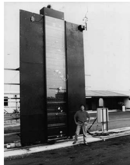
Figure 14.10 Photovoltaic blinds in a ventilated cavity
